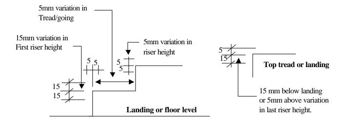
Figure 1 Tolerances in stairways
