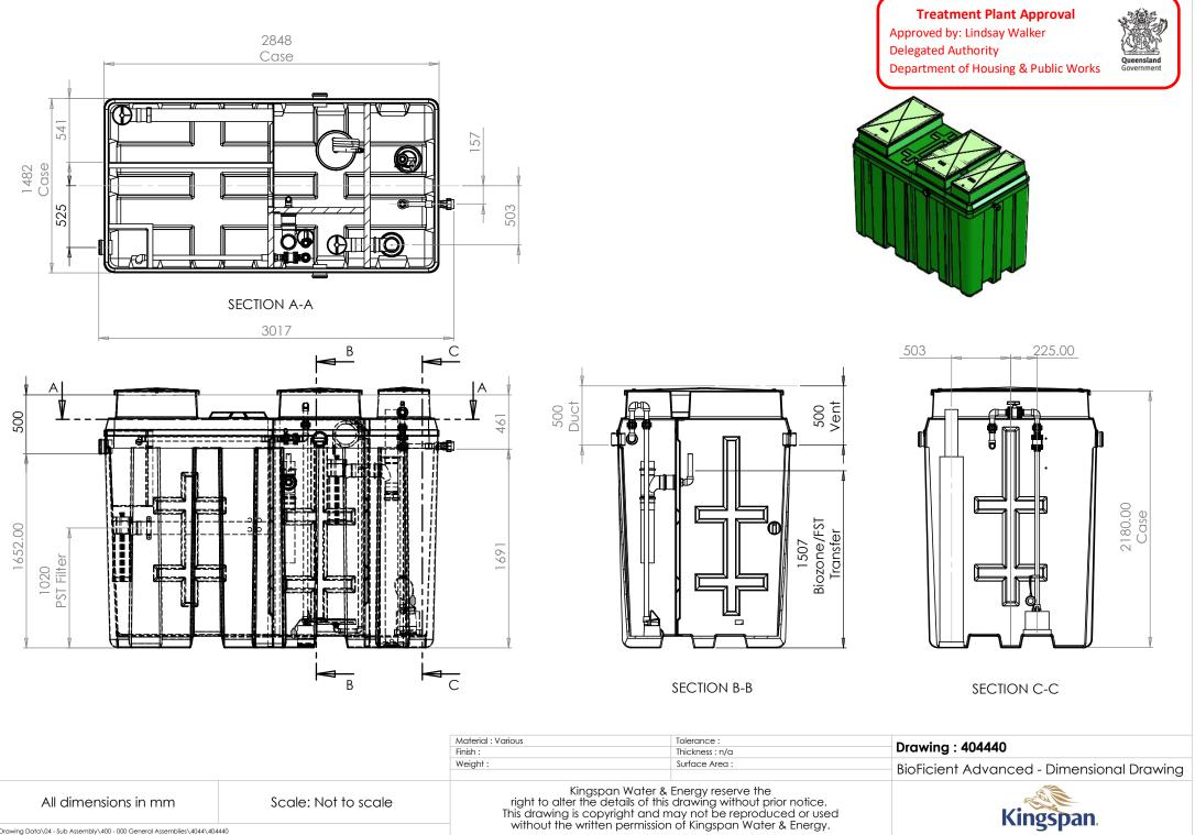
Z:\Drawing Data\04 - Sub Assembly\400 - 000 General Assemblies\4044\404440
