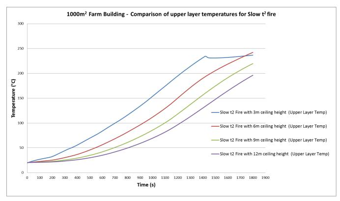
Figure 16: Smoke layer temperature for Slow t<sup>2</sup> fire within a floor area of 1000m<sup>2</sup>
