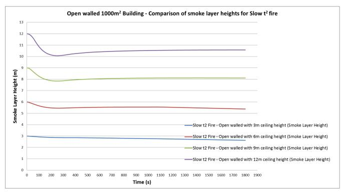
Figure 17: Smoke layer visibility for Slow t<sup>2</sup> fire within an open walled building with floor area of 1000m<sup>2</sup>
