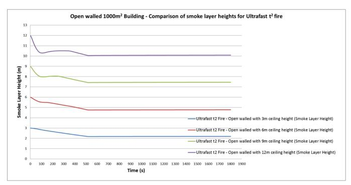
Figure 29: Smoke layer visibility for Ultrafast t<sup>2</sup> fire within an open walled building with floor area of 1000m<sup>2</sup>
