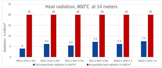
Figure 10: Heat radiation, 800°C at 14 meters
