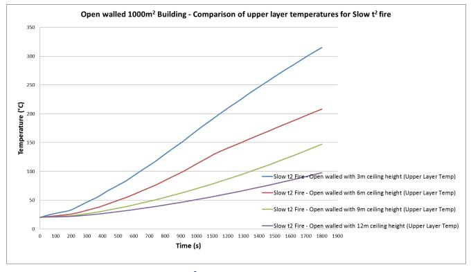
Figure 18: Smoke layer temperature for Slow t<sup>2</sup> fire within an open walled building with a floor area of 1000m<sup>2</sup>
