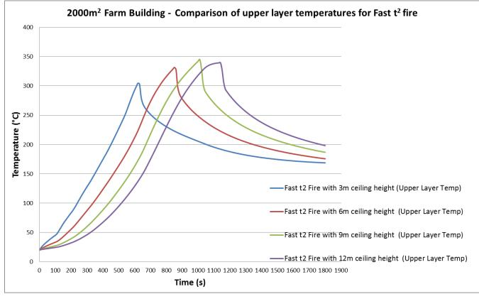
Figure 40: Smoke layer temperature for Fast t<sup>2</sup> fire within a floor area of 2000m<sup>2</sup>
