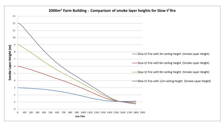
Figure 31: Smoke layer visibility for <u>Slow  $t^2$  fire</u> within a floor area of 2000m<sup>2</sup>
