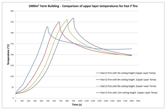
Figure 24: Smoke layer temperature for Fast t<sup>2</sup> fire within a floor area of 1000m<sup>2</sup>
