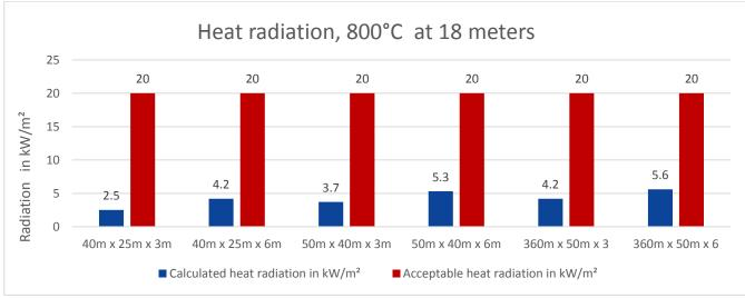
Figure 11: Heat radiation, 800°C at 18 meters
