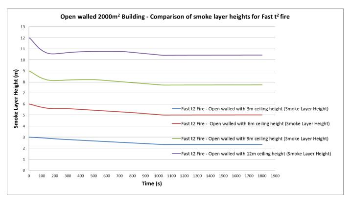
Figure 41: Smoke layer visibility for Fast t<sup>2</sup> fire within an open walled building with floor area of 2000m<sup>2</sup>
