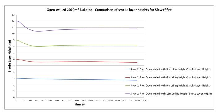
Figure 33: Smoke layer visibility for Slow t<sup>2</sup> fire within an open walled building with floor area of 2000m<sup>2</sup>
