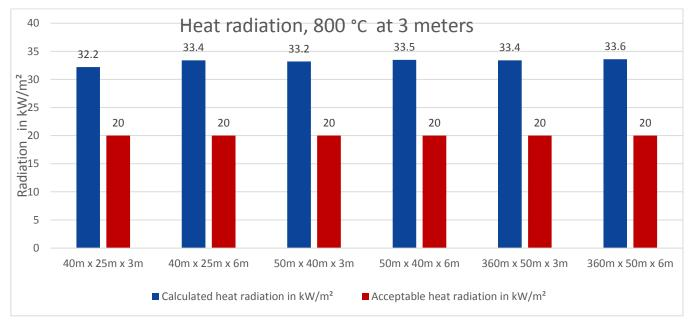
Figure 7: Heat radiation, 800°C at 3 meters
