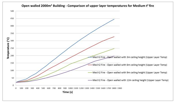
Figure 38: Smoke layer temperature for Medium t<sup>2</sup> fire within an open walled building with a floor area of 2000m<sup>2</sup>
