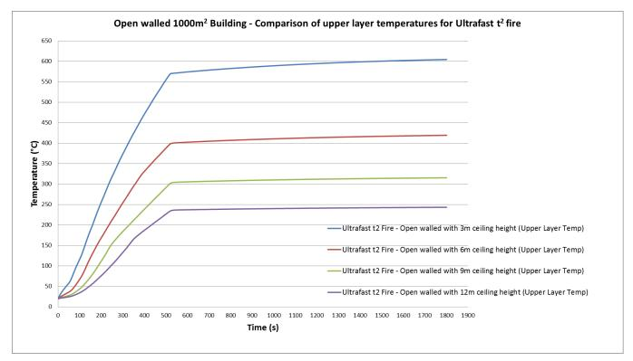
Figure 30: Smoke layer temperature for Ultrafast t<sup>2</sup> fire within an open walled building with floor area of 1000m<sup>2</sup>
