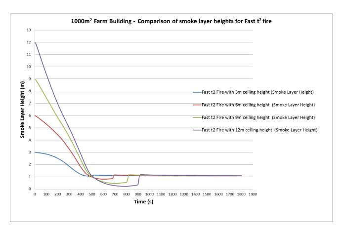
Figure 23: Smoke layer visibility for Fast t<sup>2</sup> fire within a floor area of 1000m<sup>2</sup>
