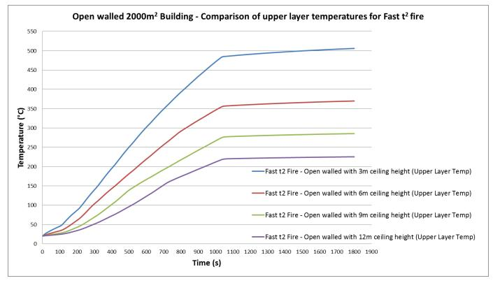
Figure 42: Smoke layer temperature for Fast t<sup>2</sup> fire within an open walled building with a floor area of 2000m<sup>2</sup>
