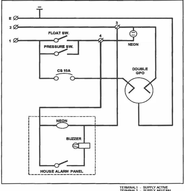
TERMINAL1 - SUPPLY ACTIVE TERMINAL2 - SUPPLY NEUTRAL TERMINAL3 - HOUSE PANEL NEUTRAL TERMINAL4 - HOUSE PANEL ACTIVE
