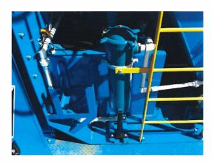
Filter Housing Assembly carries a 50 micron filter bag that is easily changed out when necessary
