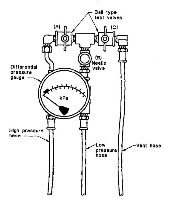
Figure 1 – Typical test kit apparatus
