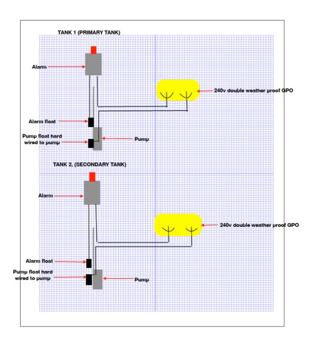
Attachment 4 – Wormsmart WSP1500PF System Schematic
