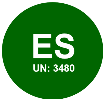
Figure 18 Indicative signage for energy storage and the battery type UN number
