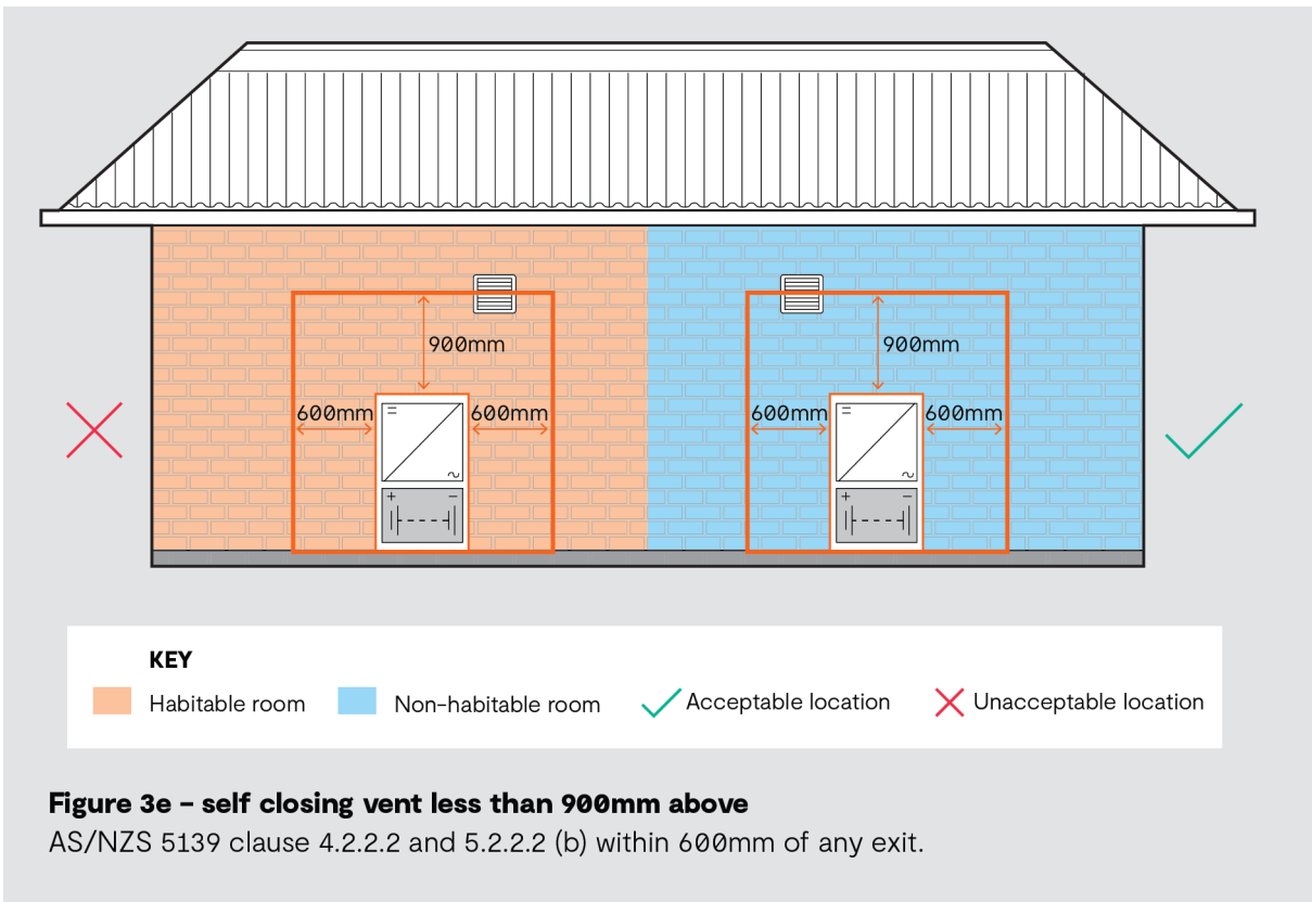
Figure 11 Battery installation clearance requirements for air vents as per AS/NZS 5139 clause 4.2.2.2 and 5.2.2.2(b)
