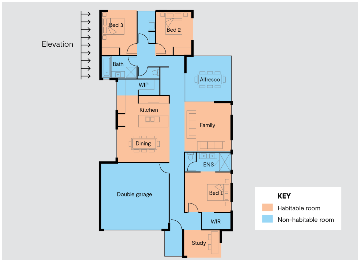
Figure 6 Examples of habitable and non-habitable rooms
