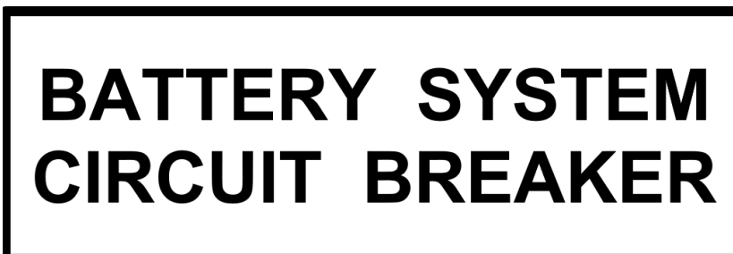
Figure 25 Indicative signage used to indicate battery system overcurrent protection
