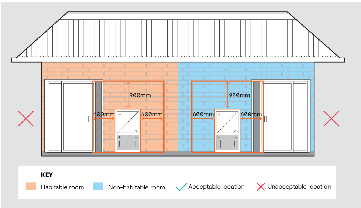
Figure 8 Battery installation clearance requirements for sliding doors as per AS/NZS 5139 clause 4.2.2.2 and 5.2.2.2(b)
