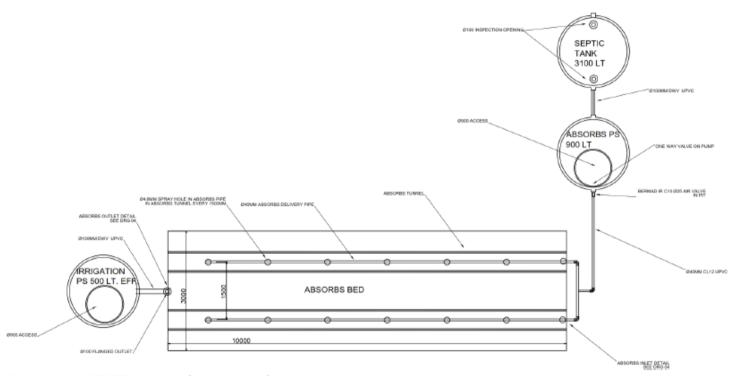
Figure 2 Typical ABSORBS™ system layout (lined configuration)
