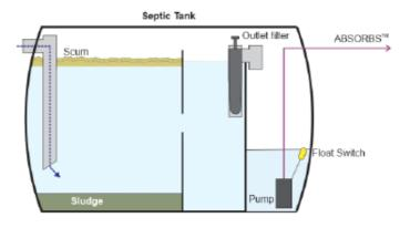
Figure 3 Schematic of your pre-treatment system
